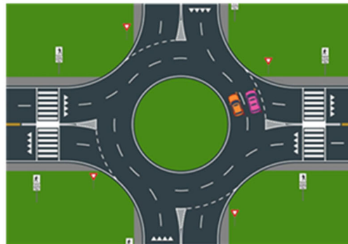
Convert intersection to roundabout (from stop or yield control on minor road)
